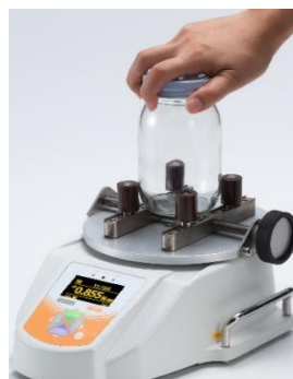
Opening/closing torque test of jar lid
