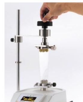
Twist test of screen protective film
